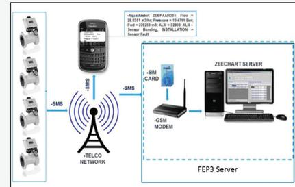
Architecture showing how DMA Meters communicate with the server to transmit data to the SCADA system
