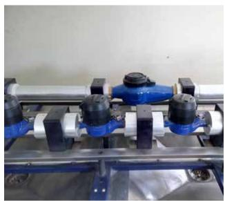
**Project** Water Meter Testing Bench
