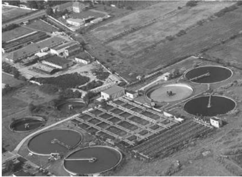
Fig 2.8 Aerobic Treatment System
